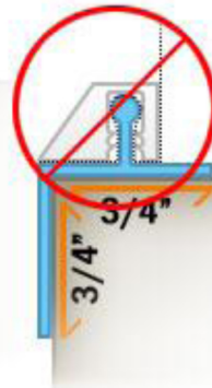
Incorrect Mount (screen is backwards)
